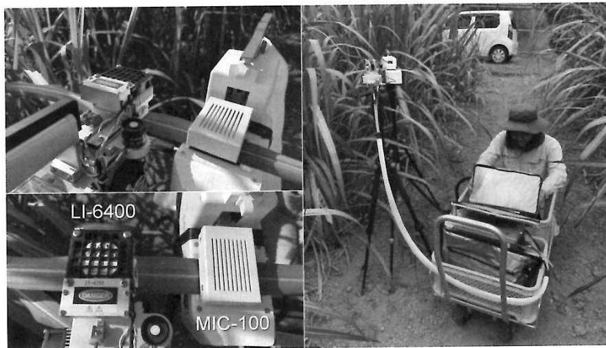
Figure 1. The outline of photosynthesis measurements using open system LI-6400 at the basal side of leaf blade and closed system MIC-100 at the tip side under field condition in Exp. 2.
